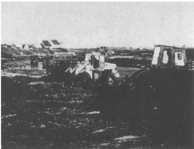
Figure 6. Front-end loaders removing oily sea weed from a beach near Portsall
